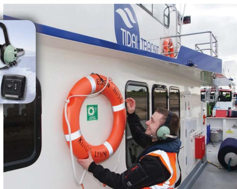
that, ease of use. The basic layout of the system typically entails a Skipper at the helm, equipped with a desk mounted microphone and speaker. As many as three mobile crew can be equipped with wireless headsets. According to the Master of the Eden Rose, no issues were encountered with the setup of the headsets. He added, "This also goes for learning how to use them. We simply donned the headsets, switched them on and they were ready to go."
