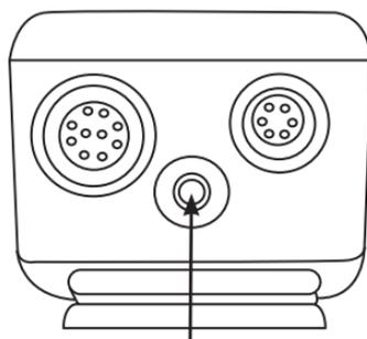
View of the top of the battery module, showing LED
