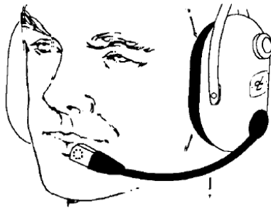
Figure 3: Microphone, Proper Position
