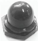
**Pushbutton Sealing Boot/Nut Assembly:** Silicone rubber (A-A-59588), 60 durometer, IP-68 protection (under normal conditions), color – black, mounting nut – nickel-plated brass (corrosion resistant), temp range: -93°F to +400°F, pressure range: 15psi (internal/external), ½-32UNS-2B bushing thread size, 0.565" button height. Resistant to salt spray, sunlight, ozone, weather, fungus and most acids and lubricating oils.
