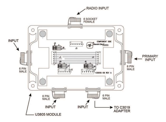
Fig. 1 - New PCB Assembly
